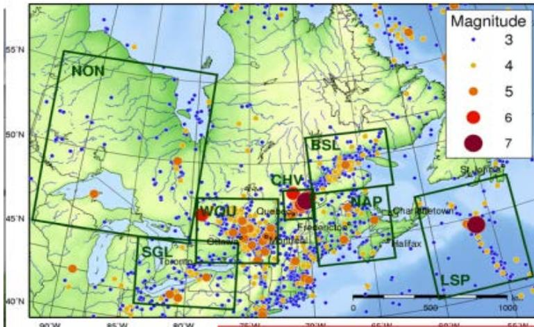
Fig. 3: Seismic Active areas in Eastern Canada – notably the Charlevoix seismic Zone in northeastern Quebec. With over 200 small earthquakes occurring each year, the Charlevoix Seismic Zone is one of the most active seismic zones in Canada.
