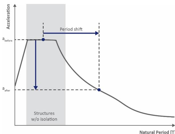
Fig. 1: Reduction of acceleration by seismic isolation only.
