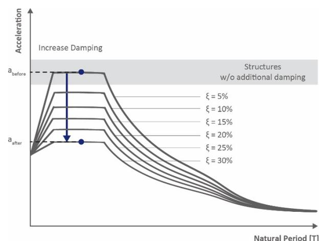
Fig. 2: Reduction of acceleration by additional damping.
